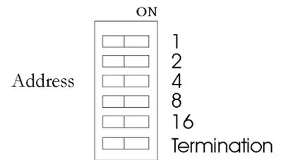
For example to select address 14, the 2, 4 and 8 switches should be pressed down to the right and the 1 and 16 switches down to the left.
