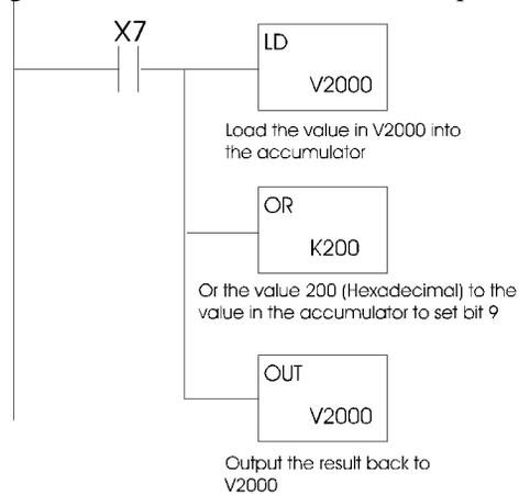
The illustration on the right is the same example for a DL305 PLC with base address 16.
