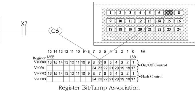
The example (below) shows a 205/405 PLC with the OM1124 configured for a PLC base address of 2000. When X7 is energized, lamp 10 will be turned on. An equivalent set of logic, using a logical AND can be used to turn the lamp off.
