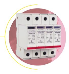
DS40 surge protectors are used mainly for primary protection of single- and three-phase networks at the main electrical panel. They provide common-mode protection (between the active conductors and ground) and are available in one-phase, single-phase, three-phase, and three-phase+neutral versions and with a remote signalling option (DS4\*S).
