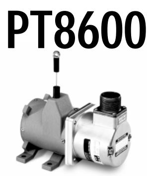
Our unique linear-to-rotational, industrial-grade motion conversion module mates to virtually any encoder, giving you a cost-effective linear position measurement solution that precisely fits your requirements. The PT8600 takes just minutes to install, fits easily into tight areas, does not require perfectly parallel alignment, and provides reliable and precise position measurements without needing periodic adjustments.
