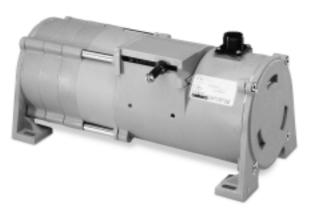
The PT9101 is a work-horse for demanding long-range applications requiring a linear position measurements in ranges up to 1700 inches. Available with either a 500, 1K, 5K, or 10K ohm potentiometer, the PT9101 operates with any basic panel meter or programmable controller.
