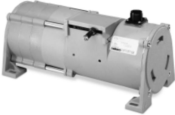
The PT9301 is a combination position and velocity transducer for demanding long-range applications requiring a linear position measurements in ranges up to 1700". A precision plastic-hybrid potentiometer provides accurate position feedback while a self-generating DC tachometer provides a velocity signal that is proportional to the speed of the traveling stainless-steel measuring cable.
