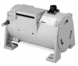
The PT9510 can operate from an unregulated 14.5 to 40 VDC power supply while providing a regulated output signal over it's full extended range of up to 1700". It provides a 0 - 10 VDC position feedback signal proportional to the linear movement of it's stainless steel measuring cable.
