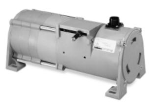
The PT9510 can operate from an unregulated 14.5 to 40 VDC power supply while providing a regulated output signal over it's full extended range of up to 1700". It provides a 0 - 10 VDC position feedback signal proportional to the linear movement of it's stainless steel measuring cable.
