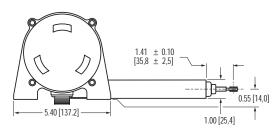
Note: Dimensions are not valid for 'increased cable tension' option. Please contact factory for correct dimensions. 6.05 ± 0.06 [153,6 ± 1,5]
