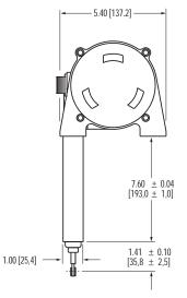
Note: Dimensions are not valid for 'increased cable tension' option. Please contact factory for correct dimensions.
