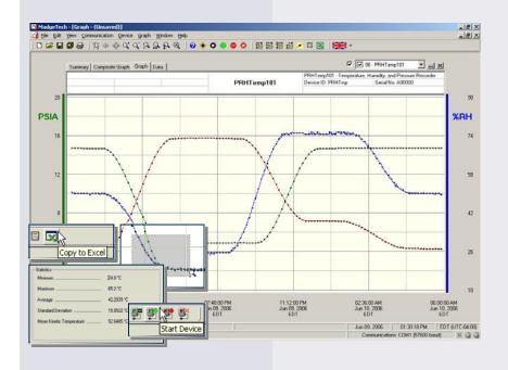
Data Recorder Software displays pressure, humidity and temperature data in an easy to use graph.
